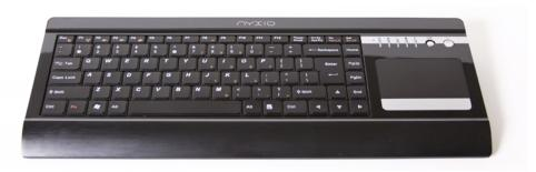
The Ascend supports WiFi for wireless network connectivity as well as a jack for connecting an Ethernet cable for wired networking. In addition, the Ascend contains a touchpad you can use to control the mouse pointer.
